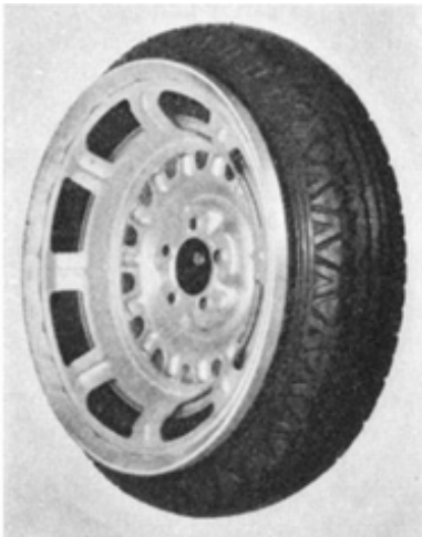
The Tire Guard, showing how it is rigidly attached to the car wheel
