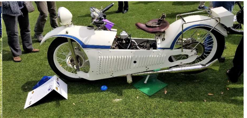
1922 Ner-A-Car, on the left, designed by Carl Neracher and made from 1918 to 1927. On the right is a 1929 Majestic built from 1929 until 1934 and this is one of ten remaining. These motorcycles were built to be as much like a car as possible. Steering was like a car and the frame was enclosed to protect the rider from "Horse Apples" and other debris.
