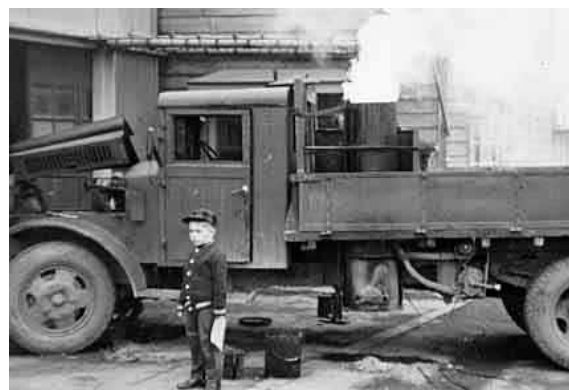
Japanese truck using coal gas to operate, circa 1949. Several Japanese vehicles still used coal gas into the early 1950's.
