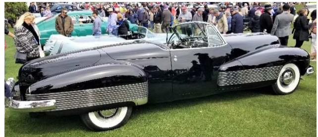
1938 Buick designed by Harley Earl and was his personal car for many years. It had a prototype 2-speed torque converter transmission. Was this the forerunner of the Dynaflo?
