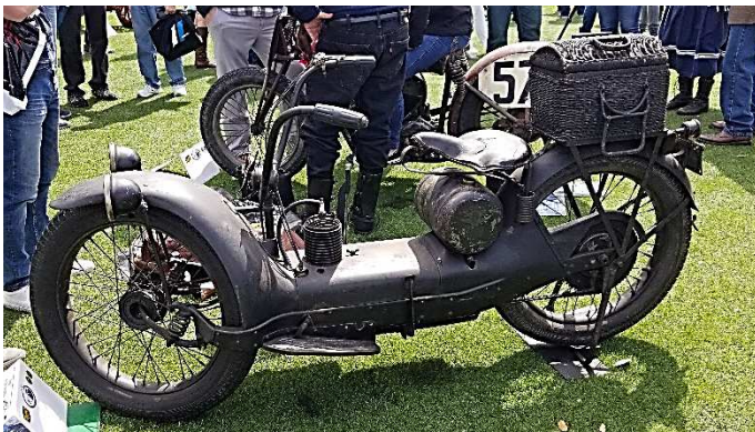
1922 Ner-A-Car, on the left, designed by Carl Neracher and made from 1918 to 1927. On the right is a 1929 Majestic built from 1929 until 1934 and this is one of ten remaining. These motorcycles were built to be as much like a car as possible. Steering was like a car and the frame was enclosed to protect the rider from "Horse Apples" and other debris.
