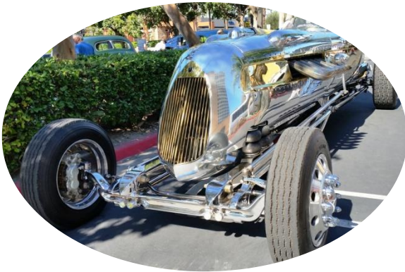
Above is what we call a "Specialty Car". It is a custom made vehicle powered by a WWII Packard Twelve Marine Engine which was used in the U.S Navy's famous PT-Boats. This engine produces over 1500 horse power
